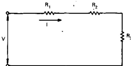
$$R_T = R_1 + R_2 + R_3$$
